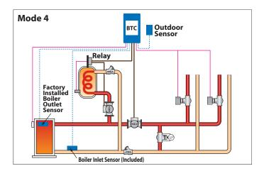
The control receives a heat demand provided from zone valve end switches or a switching relay end switch. The control turns on the boiler pump and operates the boiler to maintain the outdoor reset boiler temperature at the boiler outlet sensor. The control receives a setpoint demand from a DHW aquastat. The control turns on the boiler pump and operates the boiler to maintain the setpoint boiler target temperature at the boiler outlet sensor whenever a setpoint demand is present.
