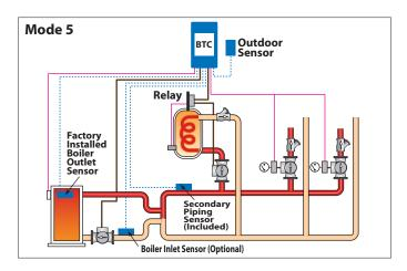
The control receives a heat demand provided from zone valve end switches or switching relay end switch. The control turns on the boiler pump and operates the boiler to maintain the outdoor reset target temperature at the boiler supply sensor. The control receives a setpoint demand from a DHW aquastat. The control turns on the boiler pump and operates the boiler to maintain the setpoint boiler target temperature at the boiler supply sensor whenever a setpoint demand is present.
