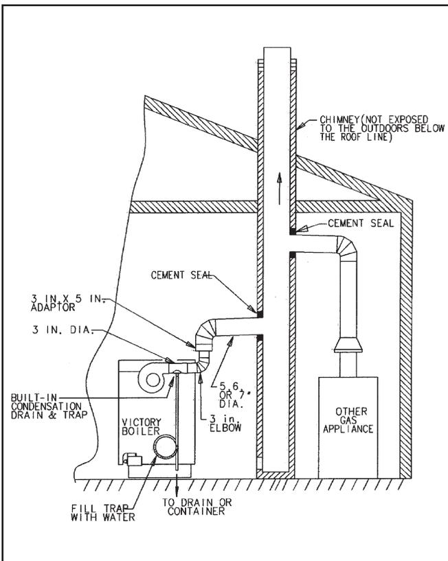
Figure 4. Chimney venting
